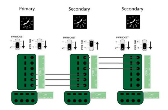
• Correct installation of Power Sharing with 4 chargers
