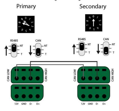
• Correct installation of Power Sharing with 3 chargers
